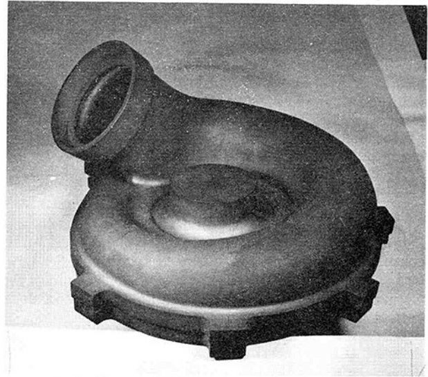
Fig. 4 Slip cast SASC turbine scroll front and backplate
